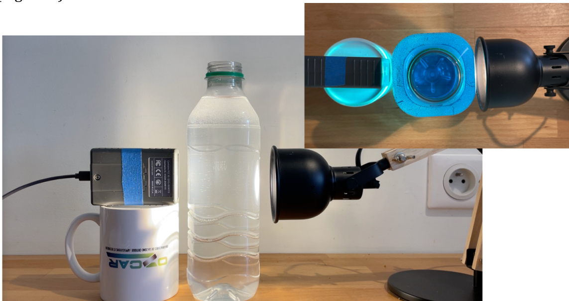
Figure 2: (Above) Experimental set-up with one-liter plastic bottle, desk lamp and light meter. Inset is view from above, after blue dye is added.
