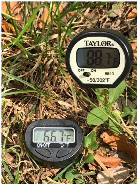
Figure 2: (Photo) Thermometer at 6" (lower L) records a soil temperature of 66.7F, while the thermometer at 1" (upper R) records a temperature of 88.7F.
