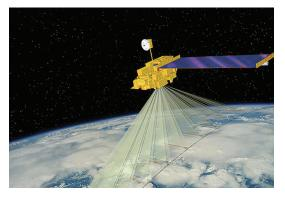
This satellite carries an instrument called MODIS that measures sea surface temperature. Credit: NASA
